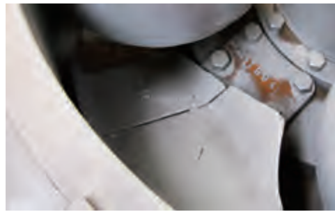
曲面可分离刀刃 Knife edge with separable curved surfaces
