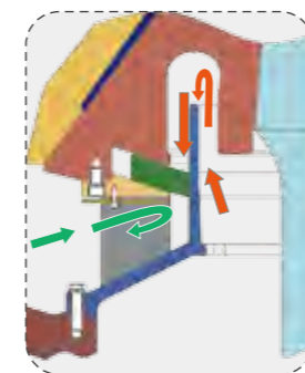
正压防尘系统 Positive Dynamic pressure air sealing
